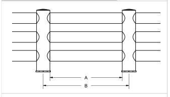
$<sup>^{\</sup>circ}$  The impact performance has not been tested for tube lengths > 1600 mm. Only use these lengths for non - critical applications.
